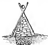
Fig. 10.—End view of half wall, on trench.
